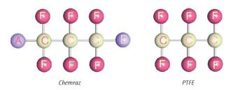
Chemraz compounds are compatible with all well fluids and gases and injection and treatment chemicals, including reservoir fluids with high H<sub>2</sub>S content, stimulation treatment fluids, completion fluids and asphaltene removers such as Xylene and Toluene together with amine-based inhibitors. Chemraz is available in O-ring, Vee ring, G-T® ring, electrical connector boots, slabs, metal bonded seals, Arlon® thermoplastic bonded seals, miniature seals, diaphragms and custom configurations.
